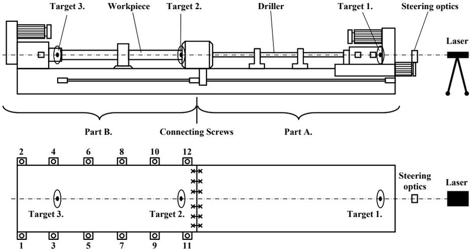
Figure 11. Schematic interpretation of deep drilling machine and measurement set-up
