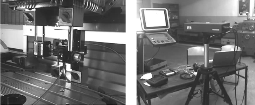
Figure 12. Real time setup for straightness measurement (left – optics, right – laser head)
