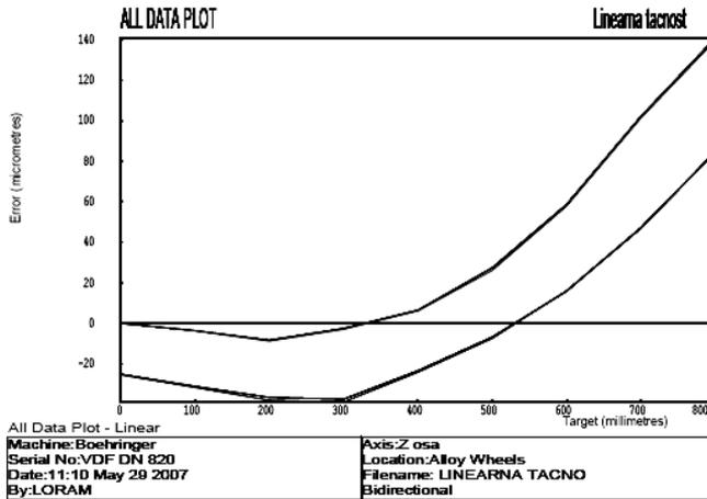
Figure 5. Results of linear displacement error measurement, CNC lathe, Z - axis
