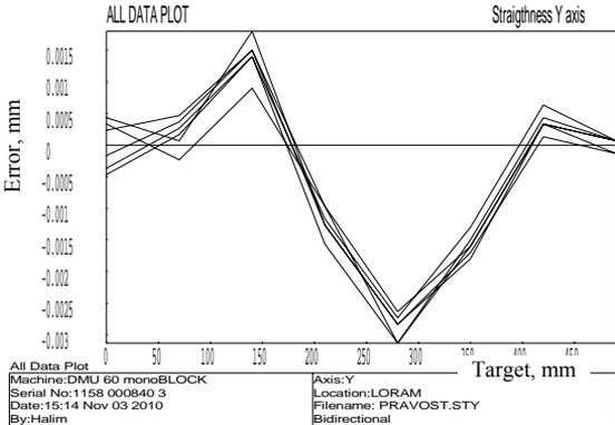
Figure 13. Graphical presentation of measurement results (Renishaw laser measurement system)
