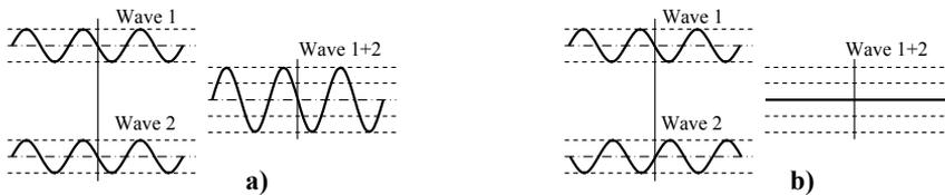
Figure 2. Constructive and destructive interference
