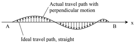
Figure 12. Definition of straightness
