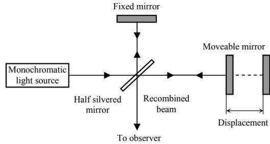
Figure 1. Basic Michelson interferometer
