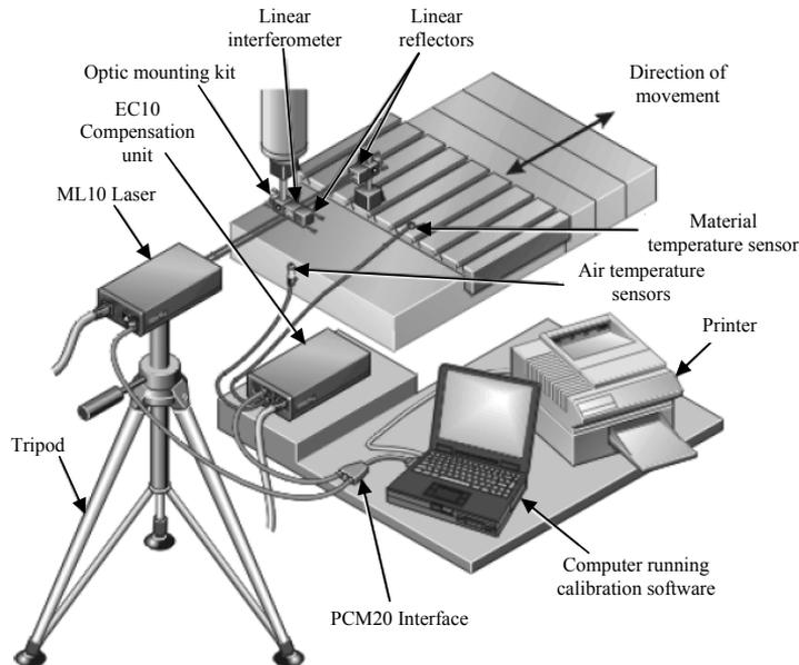
Figure 4. Typical system set-up for measuring a linear position
