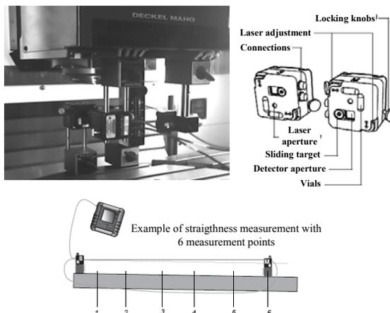
Figure 14. Damalini laser system set-up
