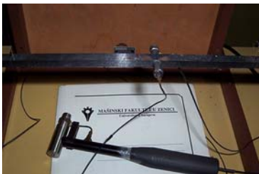
Figure 1. Impact hammer and accelerometers
