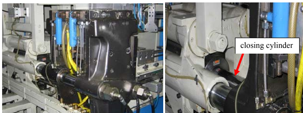
Figure 1. Closing unit together with tool (left) and closing cylinder (right)
