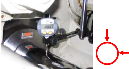
Figure 5. Motion accuracy measurement in two directions using precise gauge
