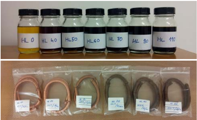
Figure 4. Hydraulic mineral oil samples after the different testing hours; different degrees of ageing and oxidation;sludge formation on copper wire
