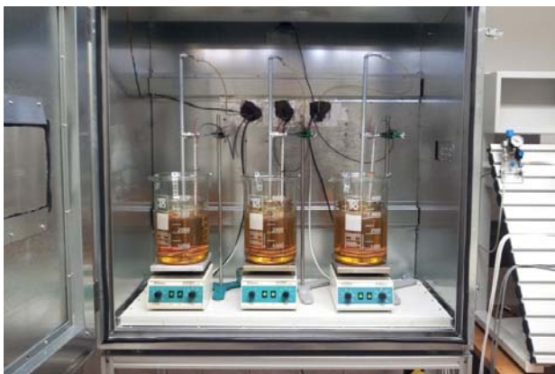
Figure 3. Thermal durability LaOH test for hydraulic oils
